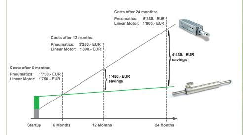
Analysis of the investment and energy costs in this application example shows that the savings from the use of an industrial linear motor, compared to the use of a pneumatic cylinder, are 1450 EUR and 4430 EUR at 12 and 24 months of service respectivelys.
